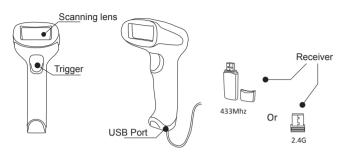
Scanner starts to work after you plug the receiver.
